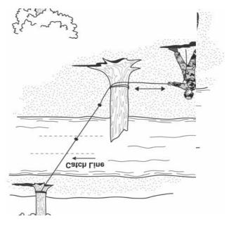
*NOTE:* The single-rope bridge must be as tight as possible so it will not sag when used.
