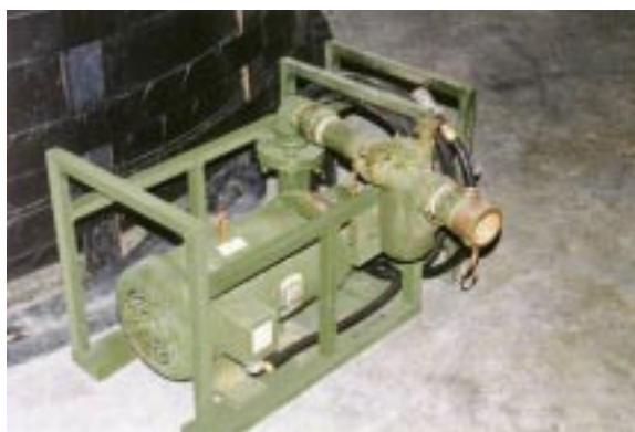
Figure 23. Backwash Pump Assembly.
