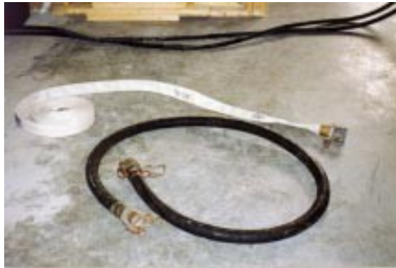
Figure 15. Suction and Discharge Hoses.
