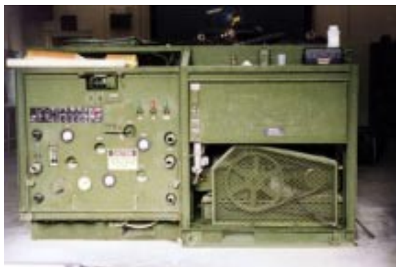
Figure 1. Reverse Osmosis Water Purification Unit.
