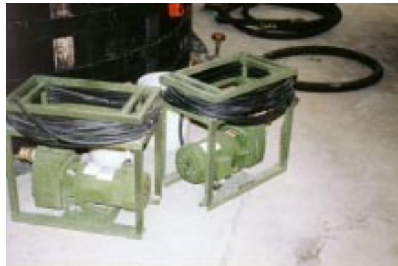
Figure 13. Raw Water Pump.
