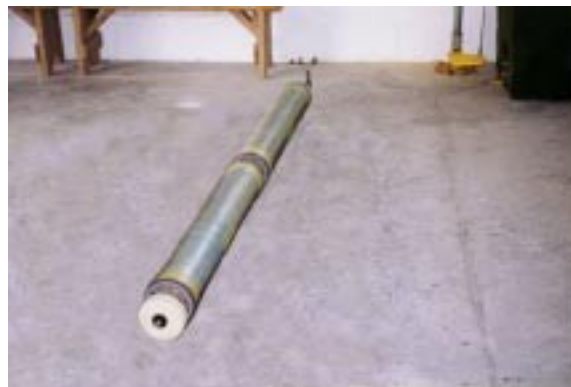
Figure 49. Puller Rod Inserted into R.O. Element String.
