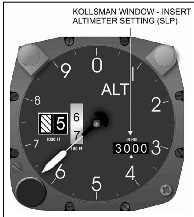
Figure 1-7 Barometric Altimeter (aka Pressure Altimeter)
