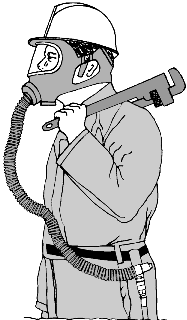
Figure 1-27.—Supplied-air respirator hose-line mask.
