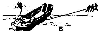
USE OF ANTIBROACHING LINES WHEN A LANDING BOAT HAS BROACHED TO PORT. NOTE THAT THE PORT LINE IS SLACK BUT KEPT WELL CLEAR OF THE SCREW. WHEN A BOAT BROACHES TO STARBOARD THE USE OF LINES IS REVERSED.
