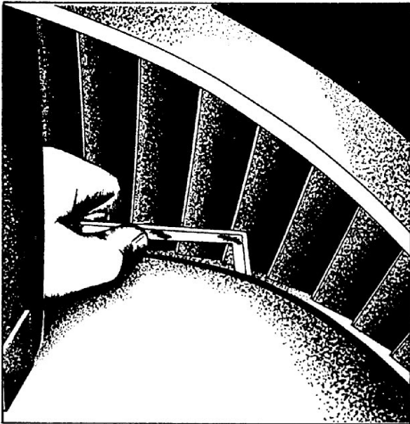
Figure 10-17.-Measuring the turbine wheel to exhaust cone clearance.
