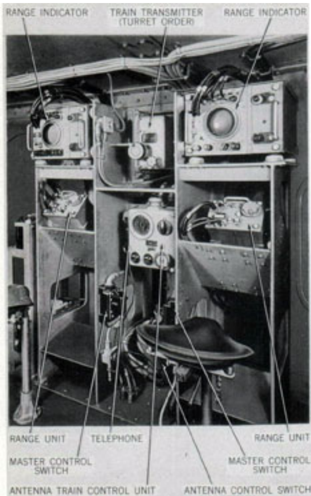
Figure 71. Radar Operator's Stations
