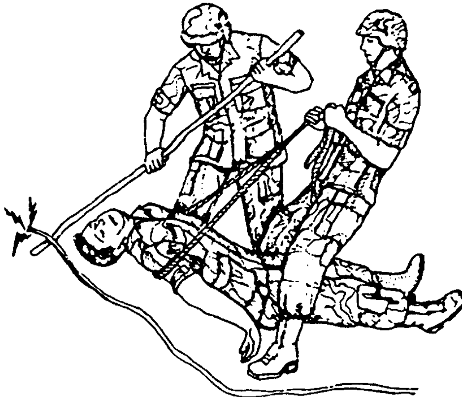
Figure 6-7. Removing an electrical wire beneath a casualty.
