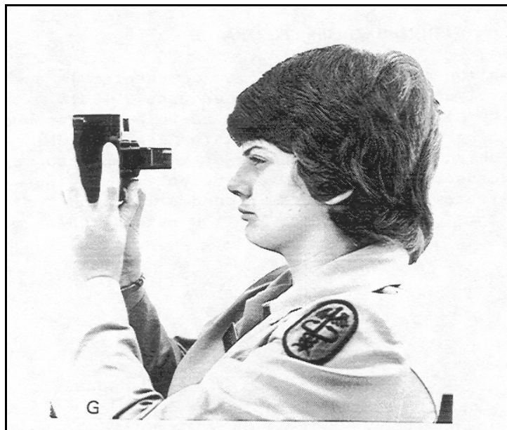
Figure 2-4. Modified OTA method, color comparator determination of free available chlorine (continued).
