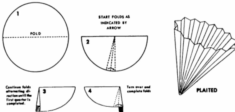
Figure 1-7. Two methods of folding filter paper.
