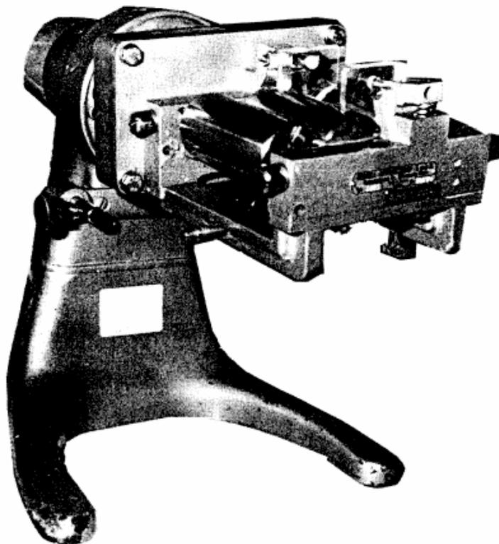
Figure 2-7. The three-roller mill (ointment mill).
