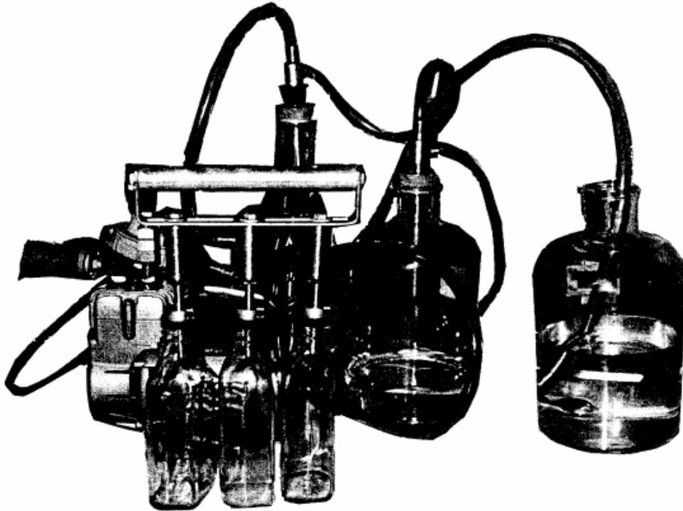
Figure 2-10. The vacuum 3 SF (suction flask) bottle filler.
