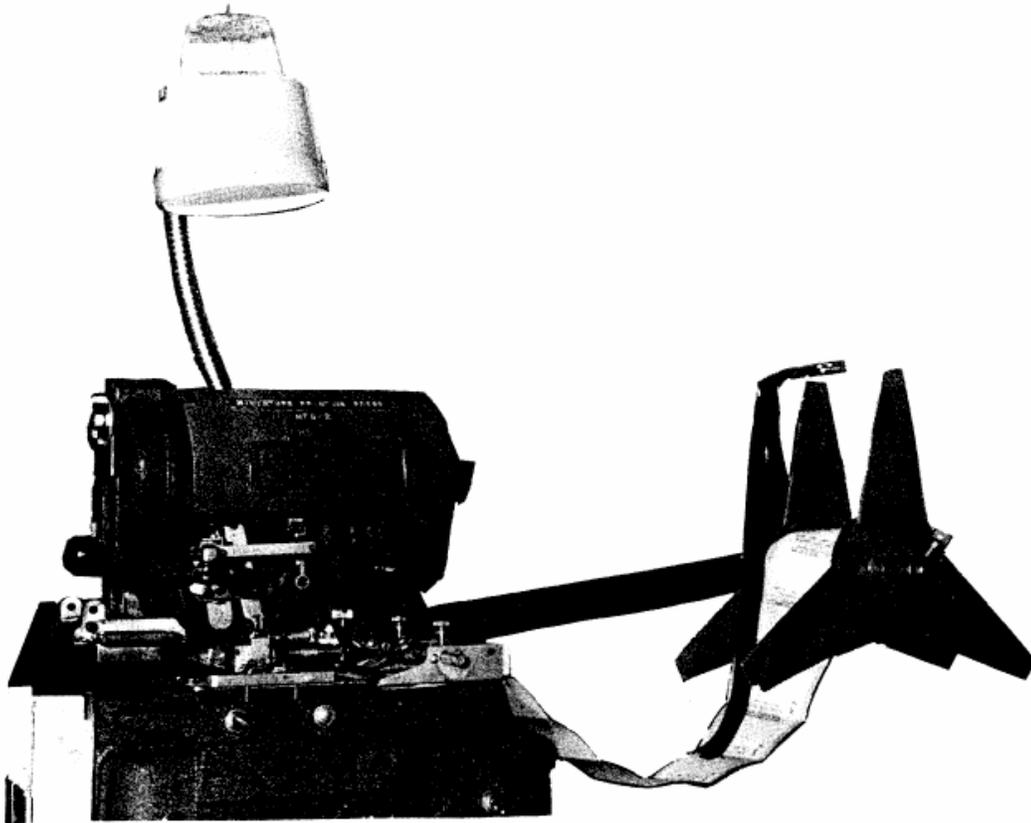
Figure 2-11. The Sobar labeling machine.
