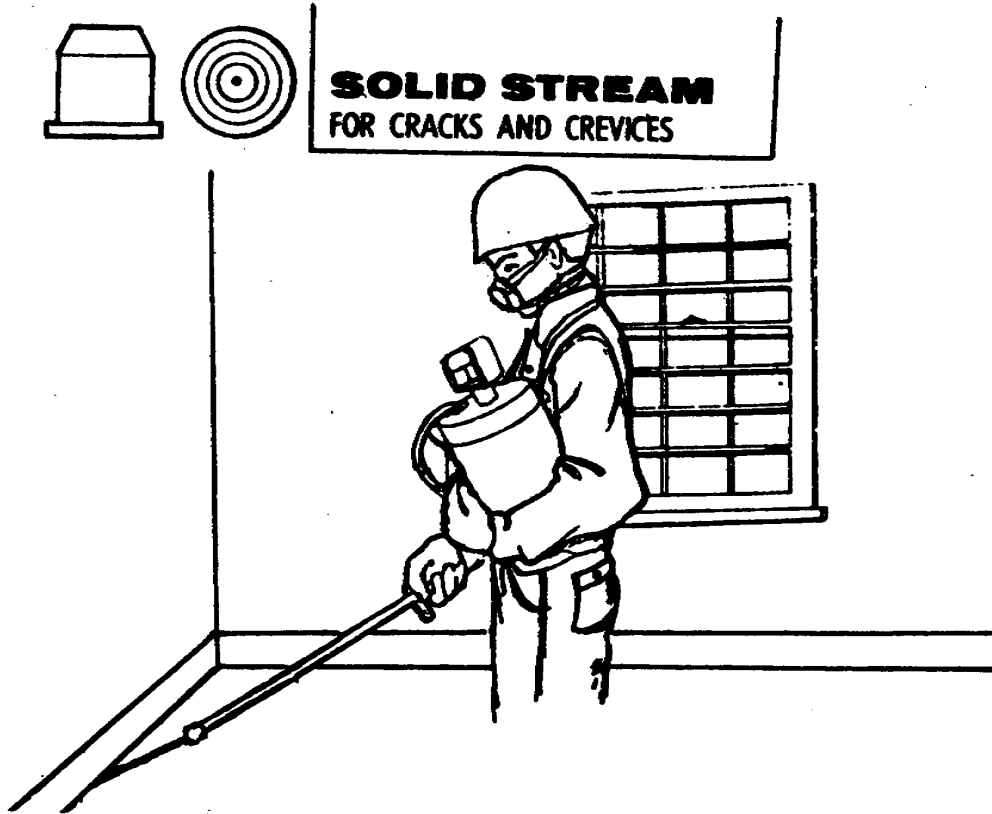
Figure 3-3. Solid stream nozzle.
