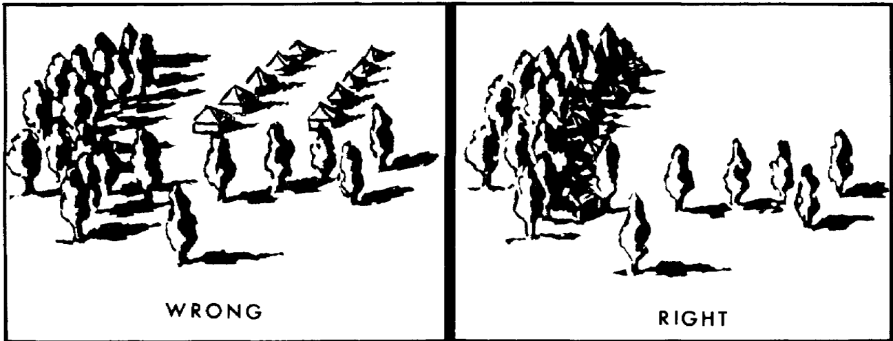
Figure 1-26. Example of Proper Siting and Dispersal of Tents in Sparsely Vegetated (Barren) Terrain).
