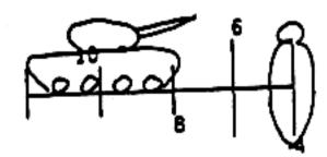
Distance to tank is 800 m Distance to 6' man is 200 m M14-M6D aiming points. Range is in hundreds of meters.
