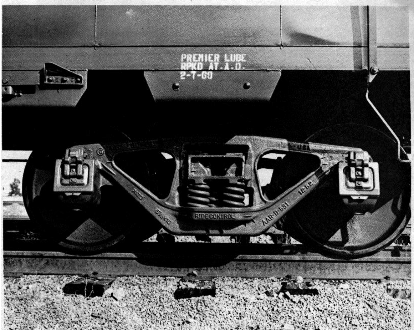
Figure 3-1. AAR standard 4-wheel, coil spring, cast bolster car truck.
