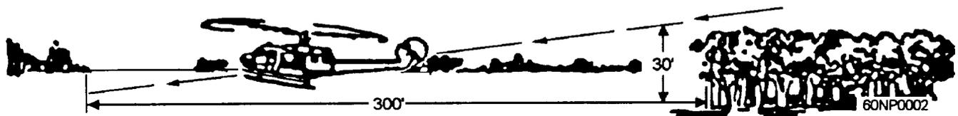
Figure 3-2.—Horizontal clearance.
