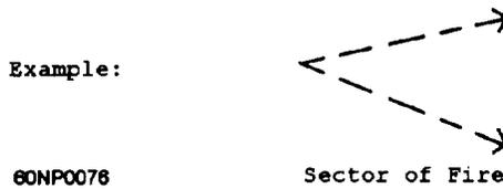
(2) A weapon symbol is normally used in conjunction with the symbol for a sector of fire. The base of the symbol indicates the weapon's position.
