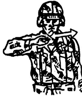
Figure 071-326-0608-31. Stop Engines
