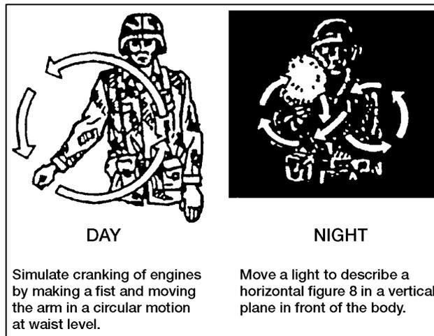
Figure 071-326-0608-21. Start Engine, or Prepare to Move
