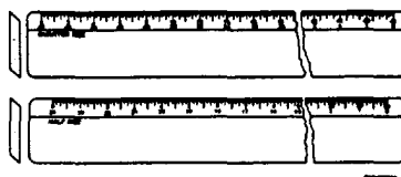
Figure 2-59. —Opposite bevel scale.
