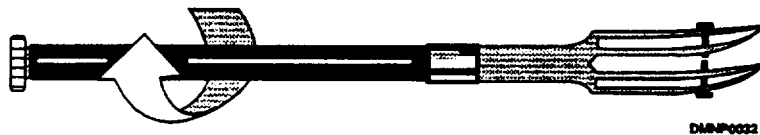
Figure 2-33. —A railroad pen with rotating handle.
