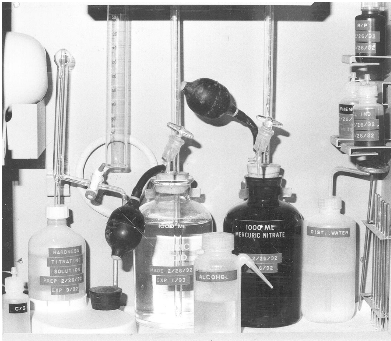
Figure 2-5.—Boiler water testing cabinet (inside view).
