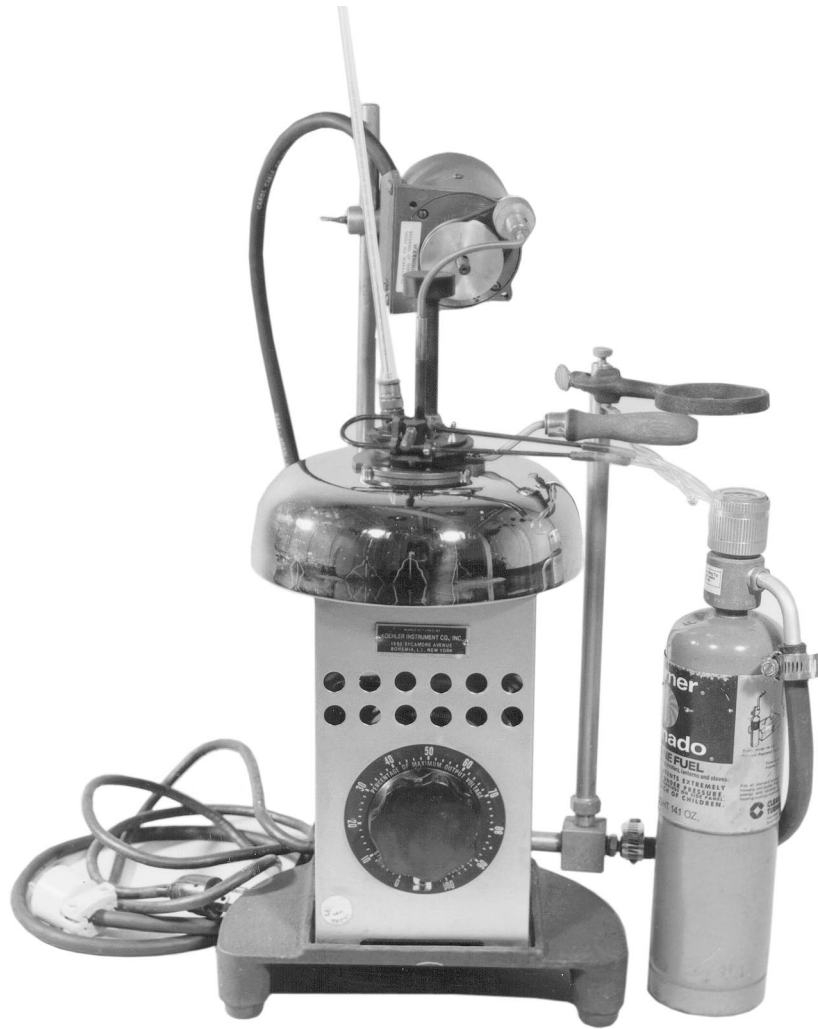
Figure 2-4.—Flash point tester.
